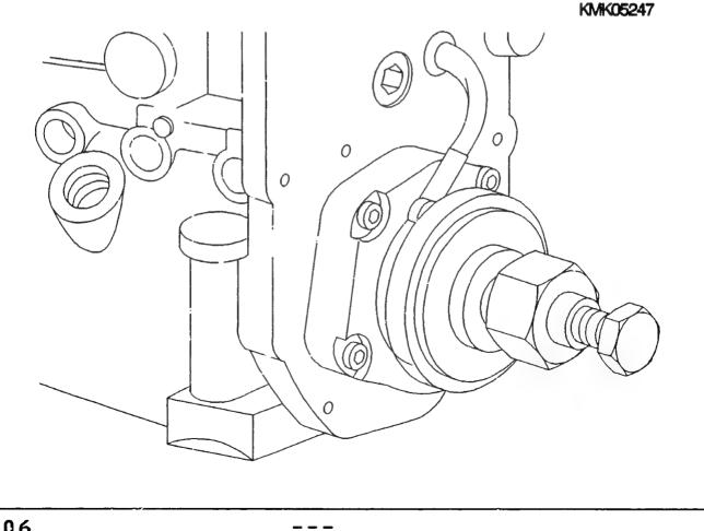
Checking position of RPS shortcircuiting ring:
